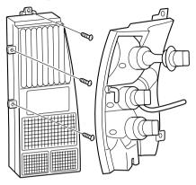
1. Open liftgate to expose the tail lamp assembly. Remove the three screws and lamp assembly from the vehicle.
